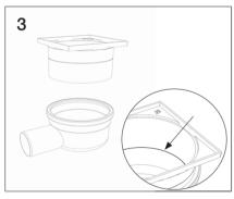
Lubricate the o-ring on the lower part properly with eg silicone paste.
